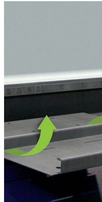
Up-and-Down function: counter folds without turning the sheet
