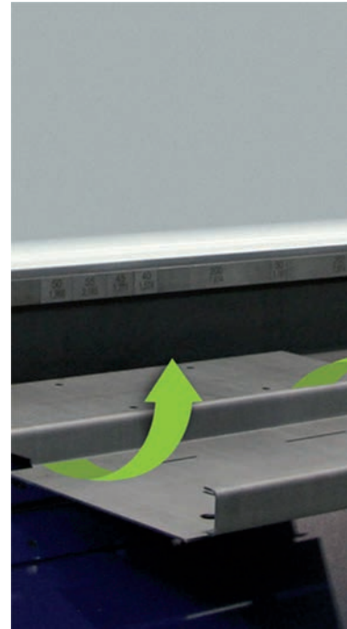
The Up-and-Down folding beam allows counterbends in one working step.
