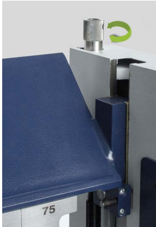
Clamping beam force adjustment
