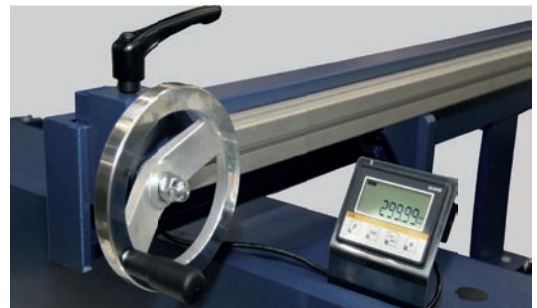
Manual back gauge, adjustable from the front, with digital readout (standard equipment)
