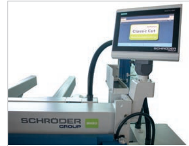
NC positioning gauge Classic Cut with touch control on turnable panel
